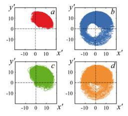
Fig. 1 Phase trajectories of the response Rössler system on the rotating plane (x', y'):  $(a) \varepsilon = 0.045$ , D = 1.5 - the phase synchronization regime,  $(b) \varepsilon = 0.037$ , D = 1.5 - eyelet intermittency,  $(c) \varepsilon = 0.045$ , D = 10 - ring intermittency,  $(d) \varepsilon = 0.037$ , D = 10 - intermittency of eyelet and ring intermittencies
