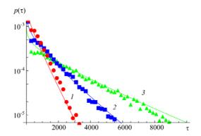
Fig. 2 Normalized distributions of the laminar phase length in the regime of intermittency of eyelet and ring intermittencies in two unidirectional coupled Rössler systems for different values of the control parameters (points) and their theoretical approximations (4) (solid lines):  $I - \varepsilon = 0.034$ ,  $T_1 = 780$ ,  $T_2 = 4500$ ;  $T_2 = 2700$ ,  $T_2 = 4500$ ;  $T_2 = 45$
