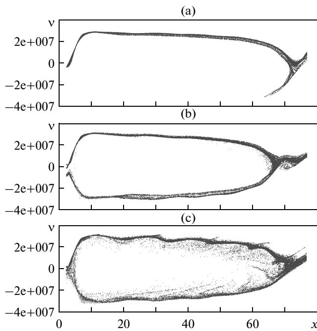
**Fig. 1.** Phase portraits of the electron flow in our low-voltage vircator: (a)  $t = 7$  ns; (b)  $t = 15$  ns; (c)  $t = 34$  ns.
