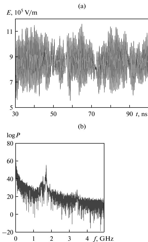
**Fig. 2.** (a) Temporal implementation of oscillations of the longitudinal component of electric field at  $x = 60$  mm and (b) its spectral composition.
