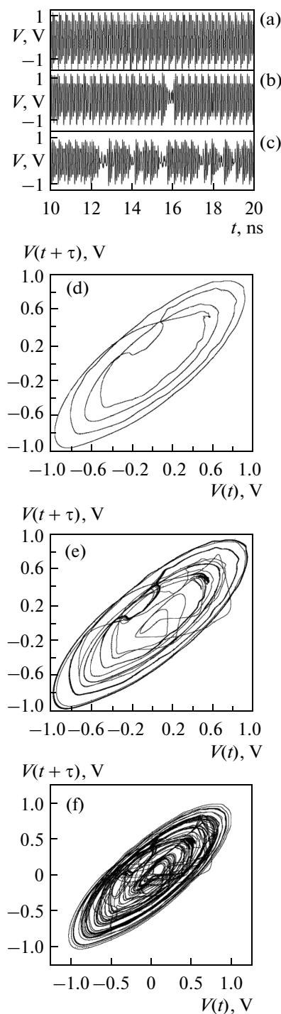
**Fig. 2.** (a–c) Time implementations and (d–f) phase portraits of fluctuations in voltage in the resonator upon a rise in power supply voltage: (a, d)  $V_0 = 844$  mV; (b, e)  $V_0 = 846.6$  mV; (c, f)  $V_0 = 848$  mV. Frequency of external resonator  $f_Q = 13.81$  GHz; quality  $Q = 150$ .
