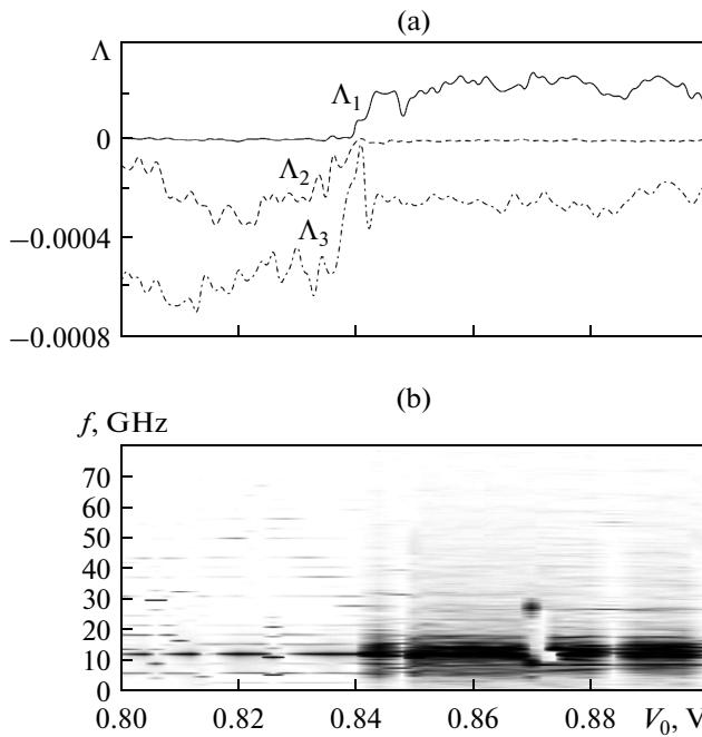
**Fig. 1.** (a) Dependences of three senior Lyapunov exponents on the voltage of the superlattice power supply. (b) Spectral composition of the voltage fluctuations in the resonator upon changes in the voltage of the power supply. Frequency of external resonator  $f_Q = 13.81$  GHz; quality  $Q = 150$ .
