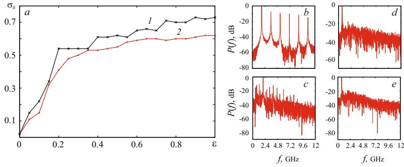
**Fig. 3.** (a) Dependencies of the synchronization index  $\sigma_s$  on the coupling parameter  $\varepsilon$  for the simply ordered chain of  $N = 10$  low-voltage vircators with slightly (curve 1) and strongly (curve 2) detuned control parameter values. (b-e) Power spectra of output signals of first (b,d) and seventh (c,e) low-voltage vircators for the different values of the coupling parameter, i.e.  $\varepsilon = 0$  (b,c),  $\varepsilon = 0.2$  (d,e).
