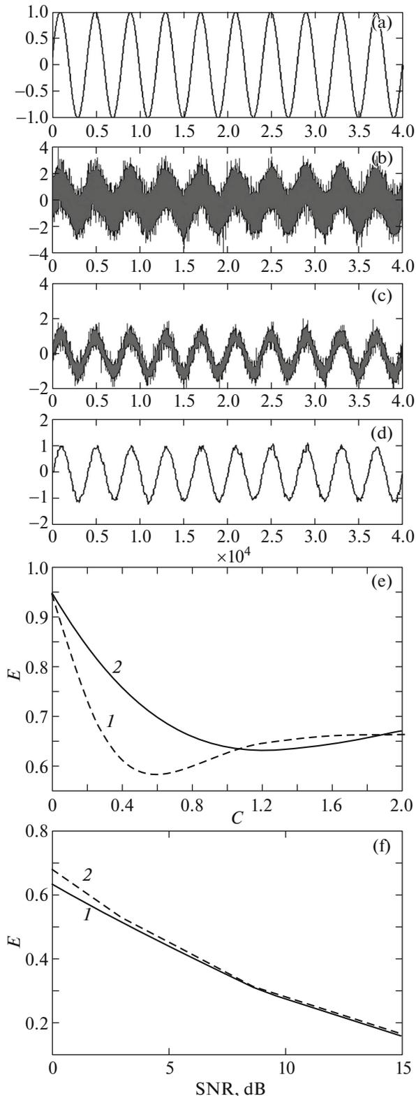
**Fig. 2.** Test-signal filtration based on a DDCWT: (a) initial signal; (b) noisy signal (SNR = 0 dB); (c, d) signal upon filtration using DWT (for the  $D^7$  wavelet basis set of the Daubechies family and DDCWT, respectively); (e, f) rms error of filtration  $E$  vs. threshold level  $C$  and SNR, respectively, as calculated for (1) DDCWT and (2) DWT methods.
