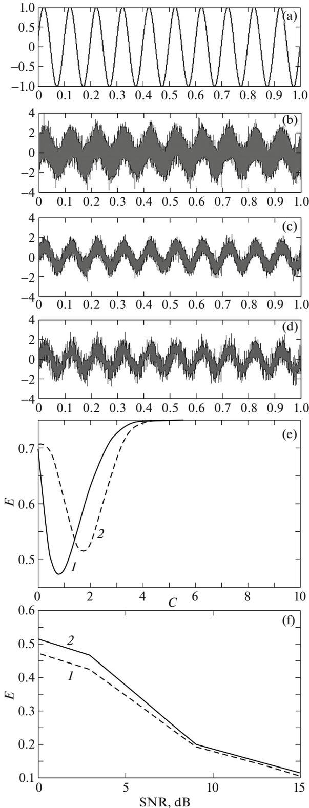
**Fig. 1.** Test-signal filtration based on a traditional DWT: (a) initial signal; (b) noisy signal (SNR = 0 dB); (c, d) signal upon filtration with soft and hard variants of threshold-function setting, respectively, for the  $D^{20}$  wavelet basis set of the Daubechies family); (e, f) rms error of filtration  $E$  vs. threshold level  $C$  and SNR, respectively, as calculated for (1) soft and (2) hard variants of threshold-function setting.
