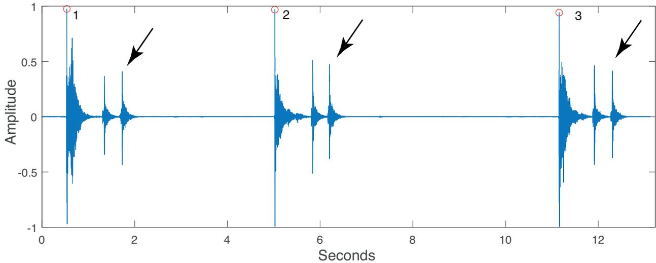
Figure 4. The signal, recorded by the capsule microphone module, for three shots. Numbers and red circles indicate the moments of the shot threshold trigger. The arrows indicate the fragments of the signal corresponding to the bolt movement of the sporting rifle during reloading.
