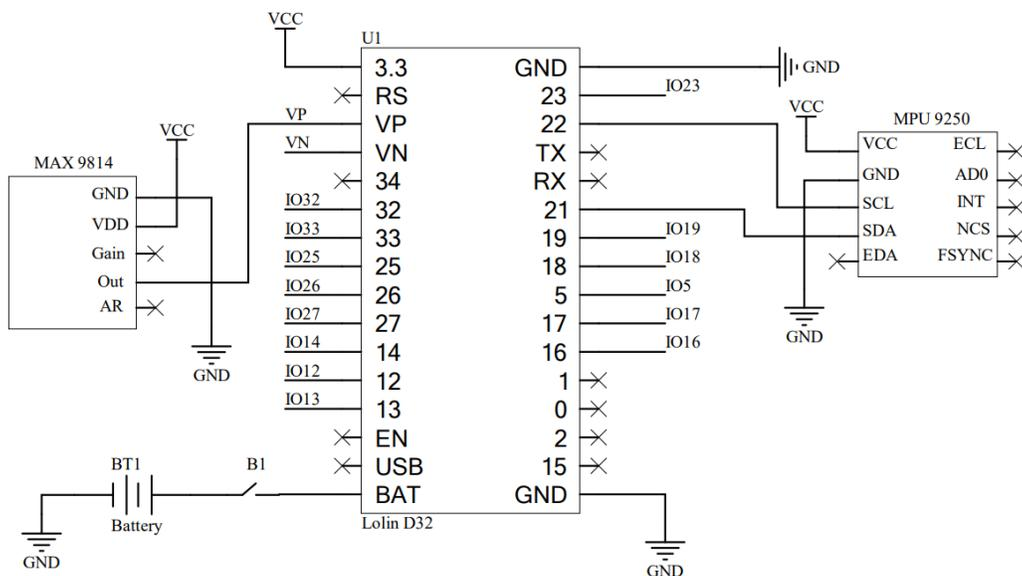
Figure 1. Schematic diagram of a portable measuring module for automatic detection of the firing moment and barrel movement during aiming. Here, MAX9814 - microphone module, MPU 9250 - inertial measuring unit, Lolin D32 - used platform based on esp32 microcontroller.
