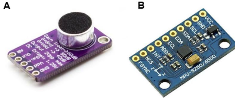
Figure 3. Sensors used in the portable tracker: a) - capsule microphone module with the built-in amplifier on the chip max9814, b) - inertial measurement unit based on the chip mpu 9250
