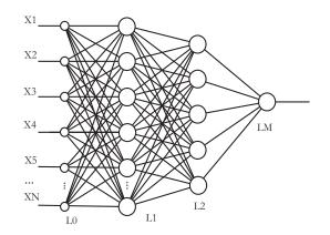
Figure 3. Structure of the Multilayer Perceptron, where  $L_0$  is the layer propagation of input signals;  $L_1$ ,  $L_2$ ,  $L_M$  are the input, hidden and output layers of the ANN respectively;  $X_1 \div X_{Nmax}$  are the EEG signal inputs ( $N_{max} = 20$ )
