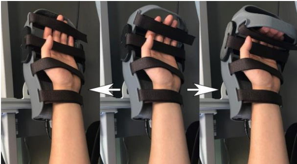
Fig. 1. Extension and flexion of fingers in the arm exoskeleton.
