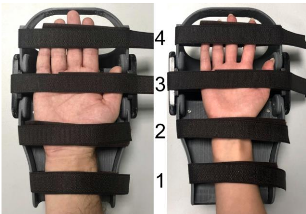
Fig. 2. Comparison of hand position for different hand sizes. The numbers indicate the numbering of the arm fixation tapes.
