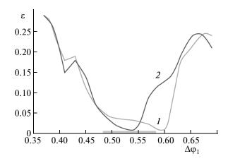
Fig. 2. GS thresholds in a system of two unidirectionally coupled low-voltage vircators on the plane of parameters  $(\Delta \phi_1, \epsilon)$  for  $\Delta \phi_2 = 0.6$  (complex-periodic regime, curve *I*) and  $\Delta \phi_2 = 0.525$  (chaotic regime, curve *2*).
