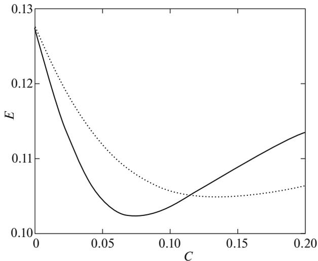
**Fig. 2.** Plots of mean-square error  $E$  of wavelet filtration vs. threshold level  $C$  for (dashed curve) DWT and (solid curve) complex wavelet transform. The variance of the normally distributed noise process added to the processed image was 0.1. DWT results were obtained with a  $D^8$  Daubechies wavelet set, which ensured minimum filtration error as compared to other basis sets of this family.
