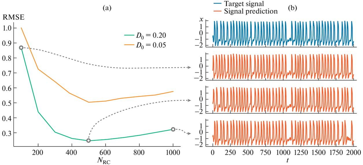
**Fig. 2.** Dependence of RMSE on the number of reservoir neurons  $N_{RC}$  during training of the reservoir computing network on the signal with noise levels  $D_0^1 = 0.05$  and  $D_0^2 = 0.2$  while predicting signals with similar noise level (a) and temporal dynamics of the FitzHugh–Nagumo stochastic neuron target signal with noise level  $D = 0.2$  and predictions of the network with reservoir size  $N_{RC}$  equal to 100, 500 and 1000 (b).
