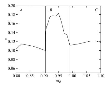
Fig. 1. GS boundary for two unidirectionally coupled Rössler oscillators [14], which reveals regions A, B, and C with different characteristic values of the coupling parameter necessary for the establishment of a GS regime (see text for explanations).
