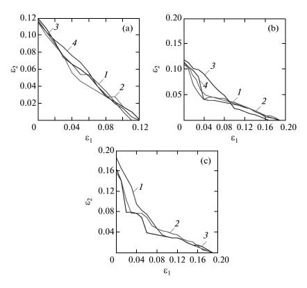
Fig. 2. GS boundaries in the system of three Rössler oscillators, plotted on the plane of coupling parameters ( $\varepsilon_1$ ,  $\varepsilon_2$ ) for various frequencies of driving subsystems:
