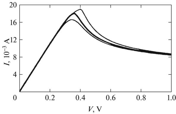
**Fig. 1.** Examples of  $I$ – $V$  characteristics for several dopant-concentration profiles at fluctuation amplitude  $D = 0.5$  (the heavy line represents the case without fluctuations).
