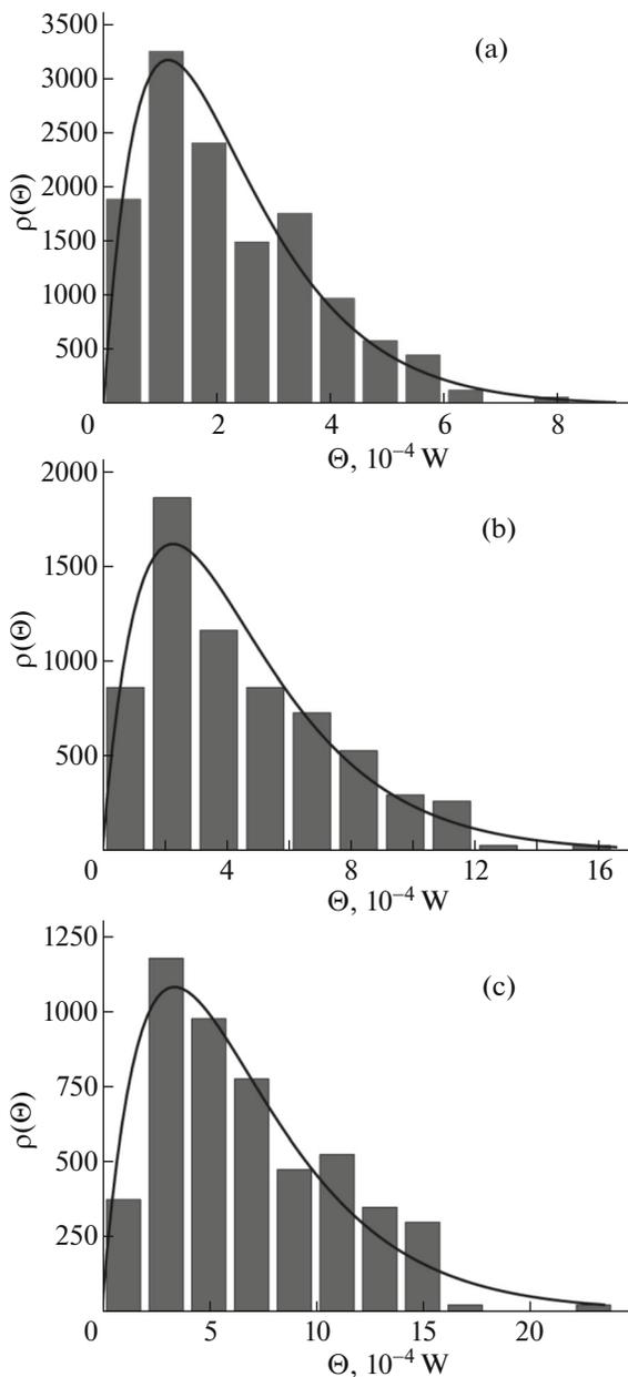
**Fig. 3.** Probability-density distributions of the integrated absolute value of the difference of currents,  $\Theta$ , for various fluctuation amplitudes  $D$ : (a) 0.25, (b) 0.5, and (c) 0.75.
