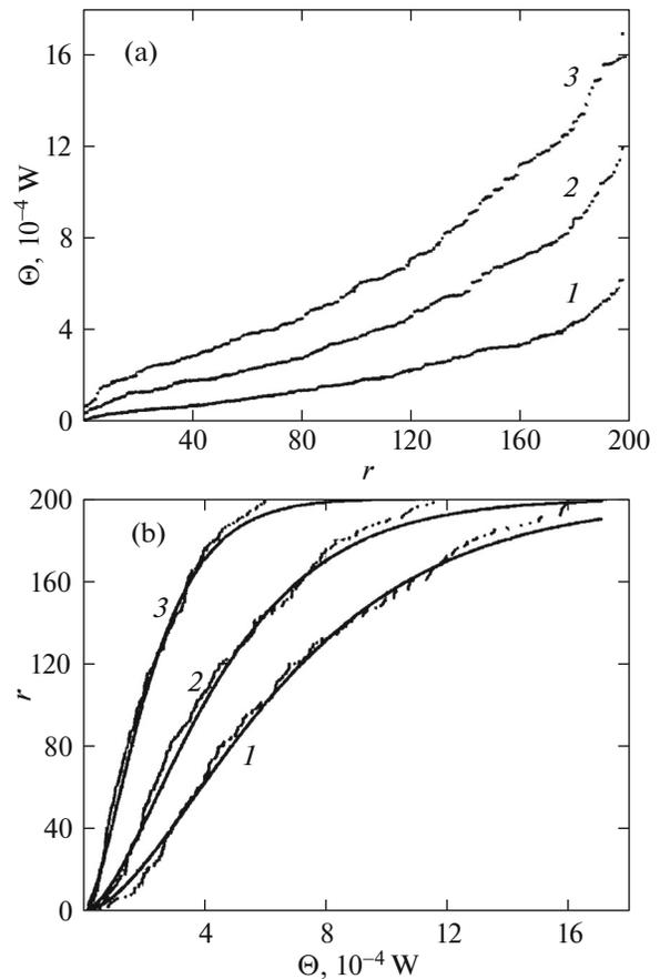
**Fig. 2.** (a) Integrated absolute value of the difference of currents,  $\Theta$ , in increasing order for various fluctuation amplitudes  $D$ ; (b) ranked distributions of the integrated absolute value of the difference of currents,  $\Theta$ , for various fluctuation amplitudes  $D$ : (1) 0.25, (2) 0.5, (3) 0.75.
