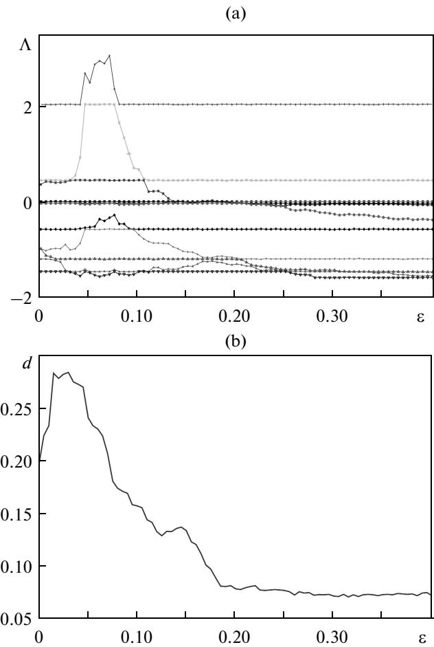
**Fig. 1.** (a) Dependence of the Lyapunov exponent spectrum and (b) measure of synchronization  $d$  on the coupling parameter in the system of unidirectionally coupled VC generators. The parameters of interacting generators are  $\Delta\phi_d = 0.5$ ,  $\Delta\phi_r = 0.4$ ,  $\alpha_d = \alpha_r = 0.9$ .
