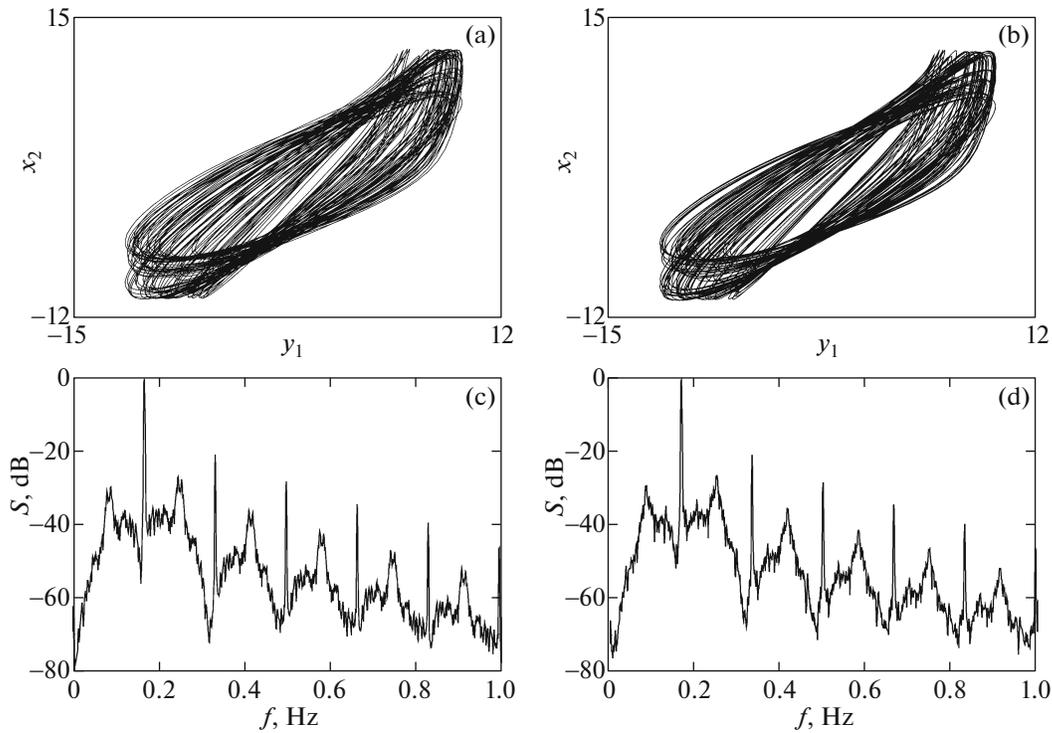
**Fig. 1.** (a, b) Phase portrait and (c, d) power spectra of (a, c) deterministic and (b, d) stochastic dynamics in the model system (1) of two coupled Rössler oscillators.
