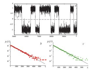
Figure 1. Time realization (*a*) and residence time distributions (b,c) for two coexisting regimes in bistable energy model Eq. (1) for b = 0. The results of numerical calculations are marked by symbols. Theoretical approximations by the regularity Eq. (6) are shown by solid lines. The parameters of approximations are (*b*)  $T_1 = 722$  and (*c*)  $T_2 = 721$ .
