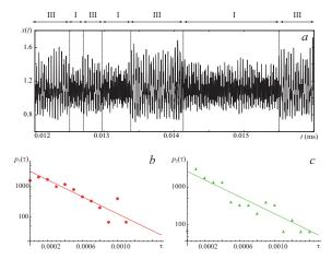
Figure 2. Time realization (*a*) and residence time distributions (b,c) for two coexisting regimes  $(b - A_1 (I), c - A_3 (III))$  in erbium-doped fiber laser Eq. (8) for noise intensity  $\eta = 0.11$  (symbols) and their analytical approximations by regularity Eq. (6) (solid lines). The parameters of approximations are  $(b) T_1 = 3.1 \times 10^{-4}$  and  $(c) T_2 = 3.9 \times 10^{-4}$ .
