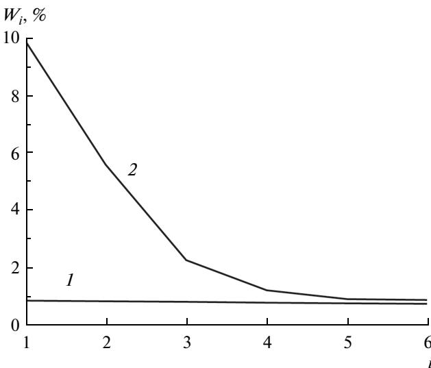
**Fig. 2.** Dependence of the energy of KL modes  $W_i$  on mode number  $i$ . Curve 1 corresponds to the formation of the reflective VC in the flow; curve 2, to the squeezed state of the beam.
